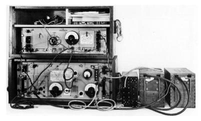
Wavemeter Class B No. 1 is comprised of Naval type Wavemeter G61 and Oscillator G35. It is powered by Wireless Set No. 11 Supply Unit Low Power No. 1
