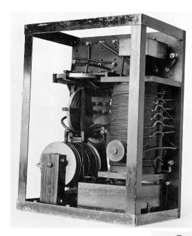
Rear view of W/T Set Field 500 watt Spark transmitter unit
