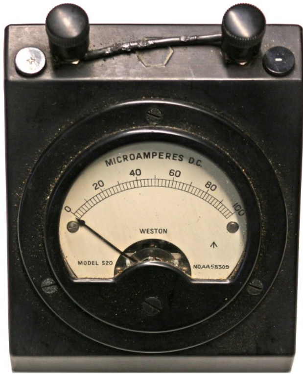
100uA meter in a Bakelite case (ZA 10495).
