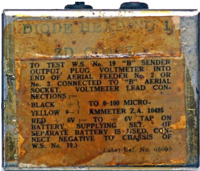
Operating instructions for the Voltmeter Valve UHF No. 1 were glued to the back side of Diode Head No. 1.
